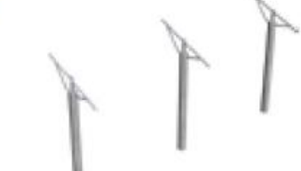
The installation of Front & Back Support and Inclined Support is done.
