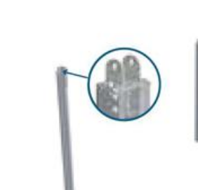
Install Post Plate onto U post
