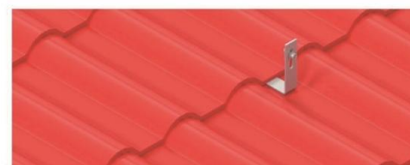
3 挂钩固定好后，将取下的瓦片复原。 After the hook is fixed, recover the tile.
