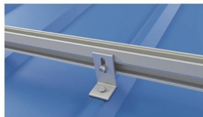
3 将导轨安装在L脚上, 并用梯形螺母固定 Install the rail on the L-foot and fix with trapezoidal nut.
